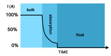
Multistage charging ensures your batteries receive optimum charging, but with minimal wear and tear, regulating the voltage and current delivered to the batteries in three automatic stages:
